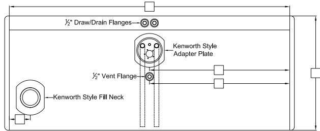
Please note: All sizes are NPTF unless otherwise noted and reference all measurements from the lateral weld seam and the end cap weld seam to the center of the fittings.
